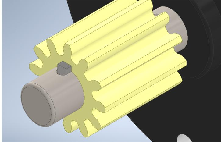
Figure 5: A pinion connected to a motor by a key, the small darker-colored part between the gear and the shaft
