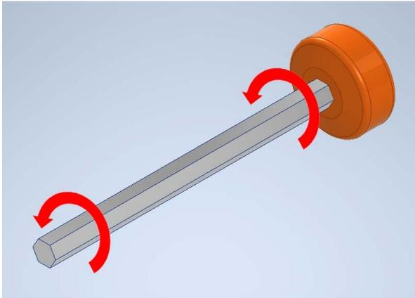
Here, the wheel and the shaft are connected in the same way, but with a hex shaft.
