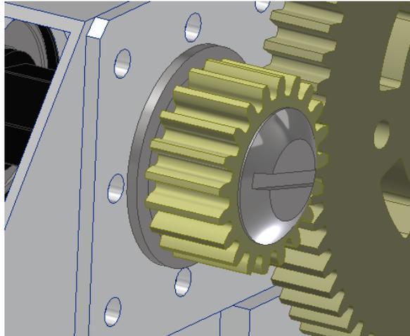
Figure 7: Sidewalk bolt in use on the 2018 robot
