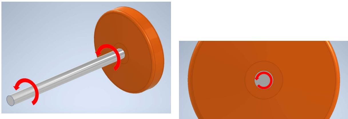
A wheel is connected to the shaft. As it rotates at one end, the other end of the shaft rotates, too.
