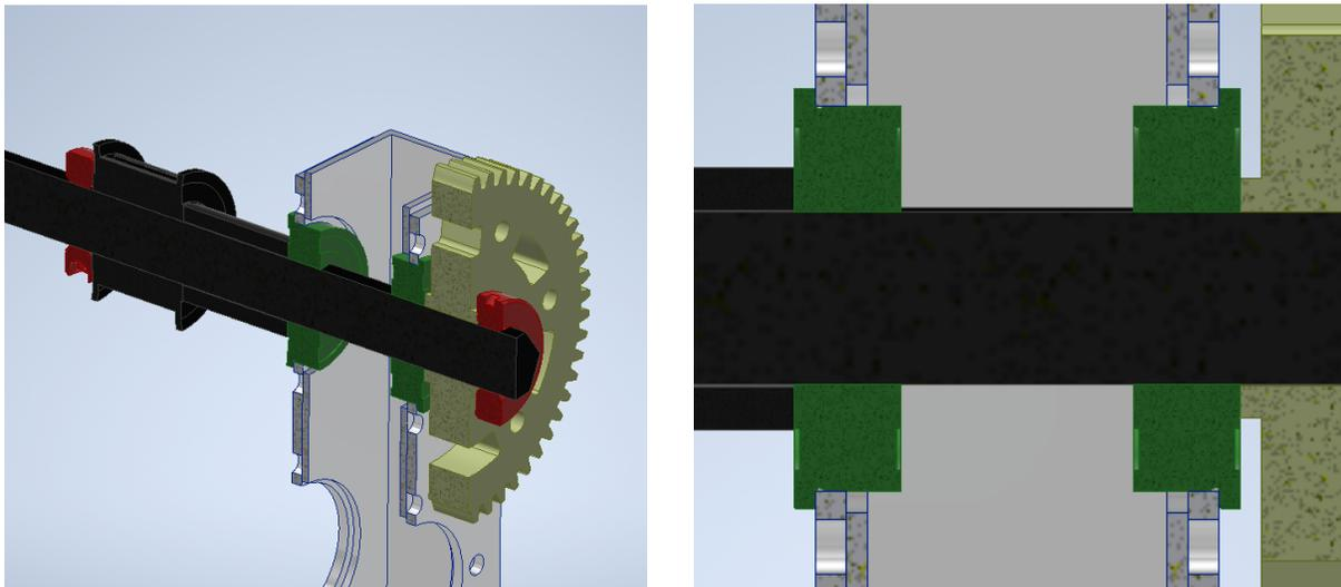
Figure 6: Section view of another shaft assembly from the 2018 robot. Here, the frame only supports the flanges in one direction, but the shaft collars on either end hold the whole assembly together so that the bearings do not slip out.
