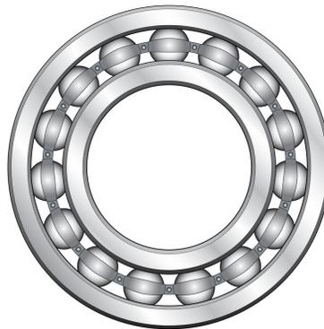
Figure 1: Diagram of a simple ball bearing
