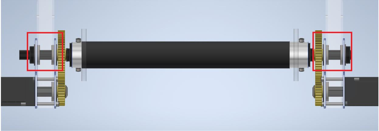
Figure 5: The climber mechanism from the 2017 robot, an example of a shaft which has more than two bearings. Here, the bearings are far enough apart that alignment is not a problem. Also, since this shaft must hold the weight of the robot, having more bearings helps distribute the weight of the robot to not put too much stress on any one bearing.
