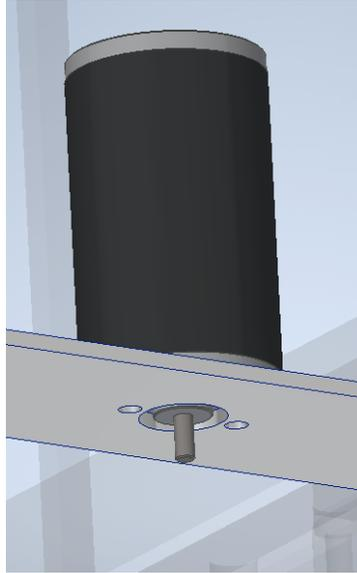
Figure 1: A BAG motor mounted to a flat bar on the 2019 robot. The holes are for bolts which are not modelled, and a pulley on the output shaft is hidden.
